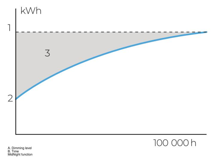
The MidNight function feature allows an autonomous dimming without the need for an additional control line. The output levels can be set to 0% (OFF) or between 10% and 100% in steps of 1%
